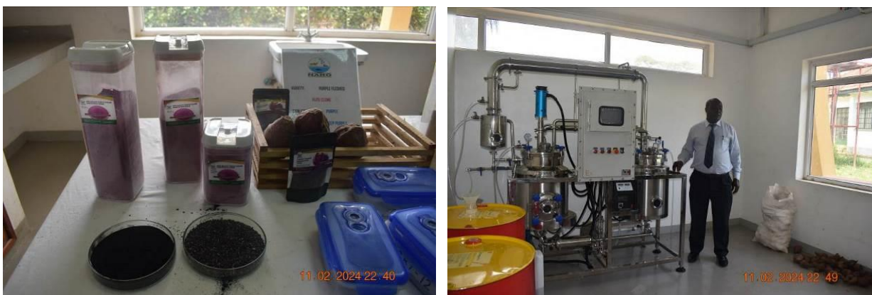
L-R: Black charcoal technology in round dishes and sweet potato powders in jars under incubation and anthocyanin mini-extractor
