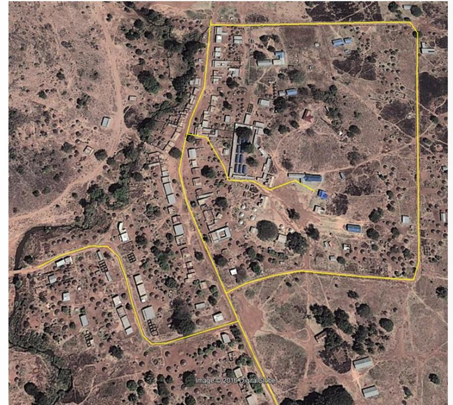
Aerial view of Agoro Subcounty, one of the villages to be electrified. The yellow line shows the proposed electricity grid distribution structure, connecting all building with in reach of the grid.
