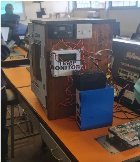
A silver fish solar dryer prototype made by UICT students
