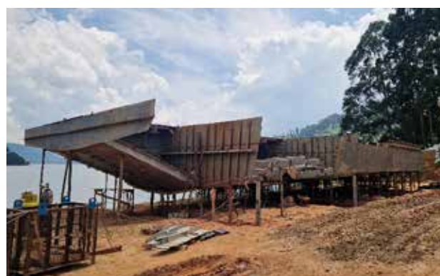
R: Lake Bunyonyi Ferries: Assembly of Ferry 1 hull
