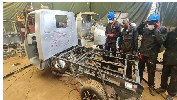
Left: The localized Kayoola EVS Frame at the KMC vehicle plant in Jinja. Right: Fabrication of the 3-in-1 Trike prototype at KMC office in Ntinda
