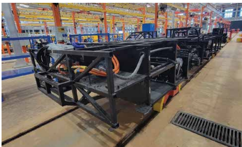
A bus chassis being assembled at the Kiira Vehicle Plant in Jinja
