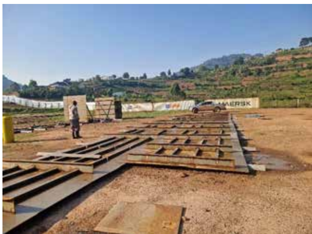
Ongoing fabrication of hull superstructure panels for Lake Bunyonyi ferries in Rubanda District
