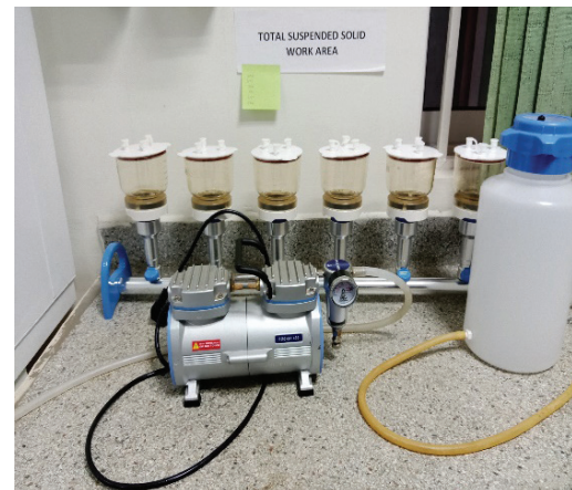
An autoclave; incubator; and Multi-Branch Manifold and Filtration Unit in the Mbale Regional Laboratory
