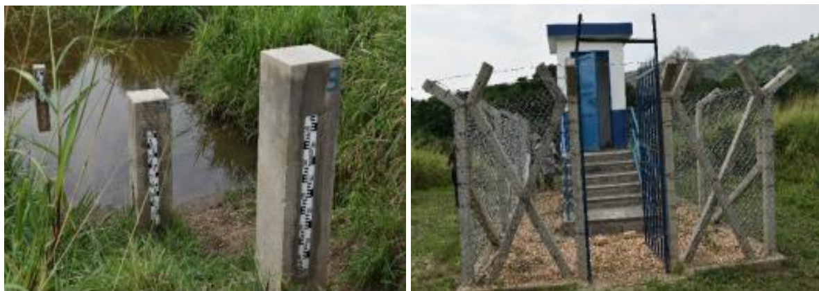
L-R: The River gauges and surface monitoring station at River Mpanga in Kitagwenda District
