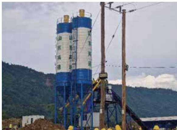
Namagumba–Budadiri–Nalugugu Road, L-R: Rock filling of a swamp section at km 7+475; concrete plant assembled at the contractor's camp in preparation for concrete works
